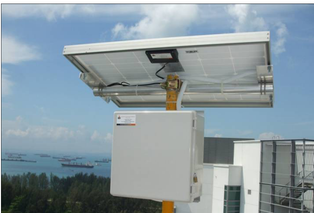
Photo 2.3.3b: Use of solar panel to power the noise meter.
