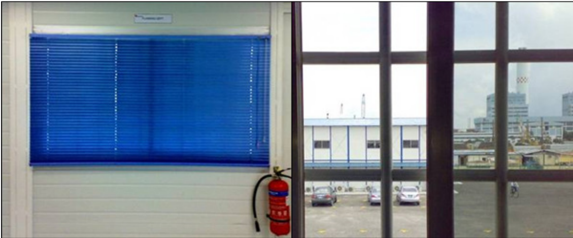
Photo 4.1.1e: Use of blinds and application of UV films on windows will help to reduce the heat transmitted into the site office. Thus less energy is needed to cool the site office.
